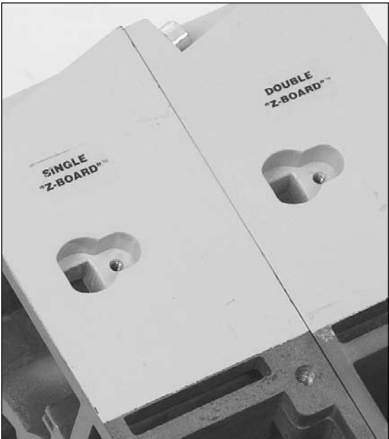
Label on manifold block indicates installed--- "Z-Board"™ type.
